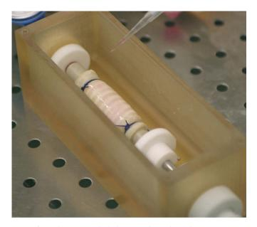
Fig. 3. The matrix inside the bioreactor during the seeding process.
