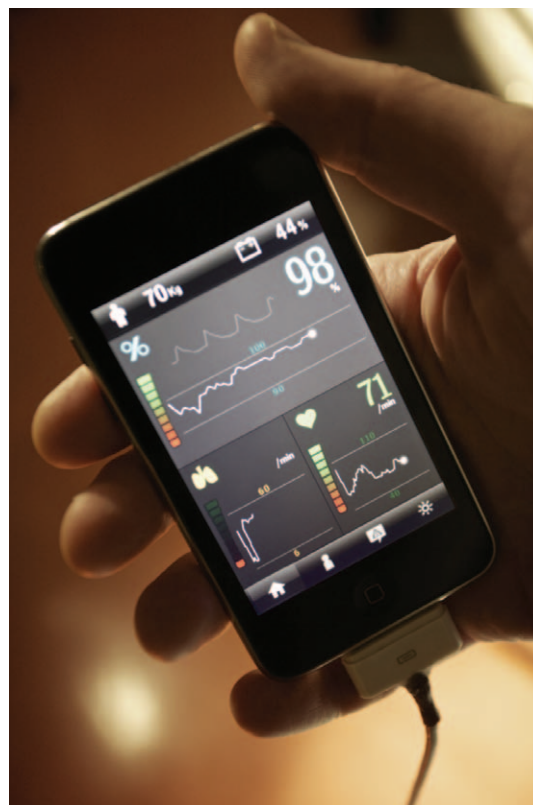
Figure 4. An example of a sensor attached to a mobile phone for pulse oximetry monitoring. This application is called the Phone Oximeter. The sensor is attached to the phone using the power port of the device.
